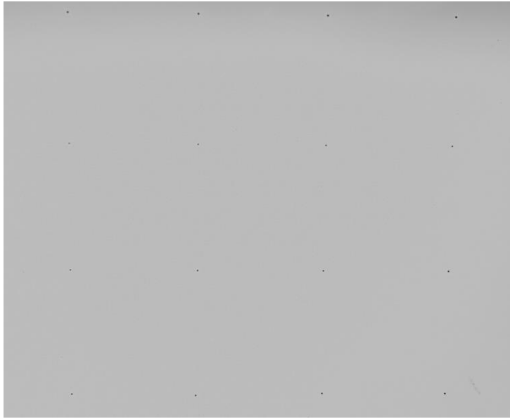
View through vacuum glazing with square ceramic supports (source: Peter Sønderkær, VELUX)
